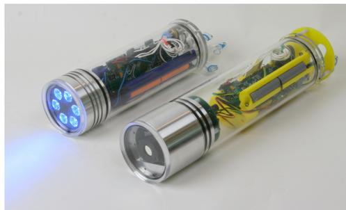
Fig. 1: The receiver and transmitter of AquaOptical.
